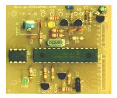
Through configuration software, the user is able to customize callsigns and other parameters. An on-board memory stores configuration information indefinitely and configuration software can be run as often as needed to change settings. The on-board voltage regulator accepts power from an unregulated 7-30 VDC source.
