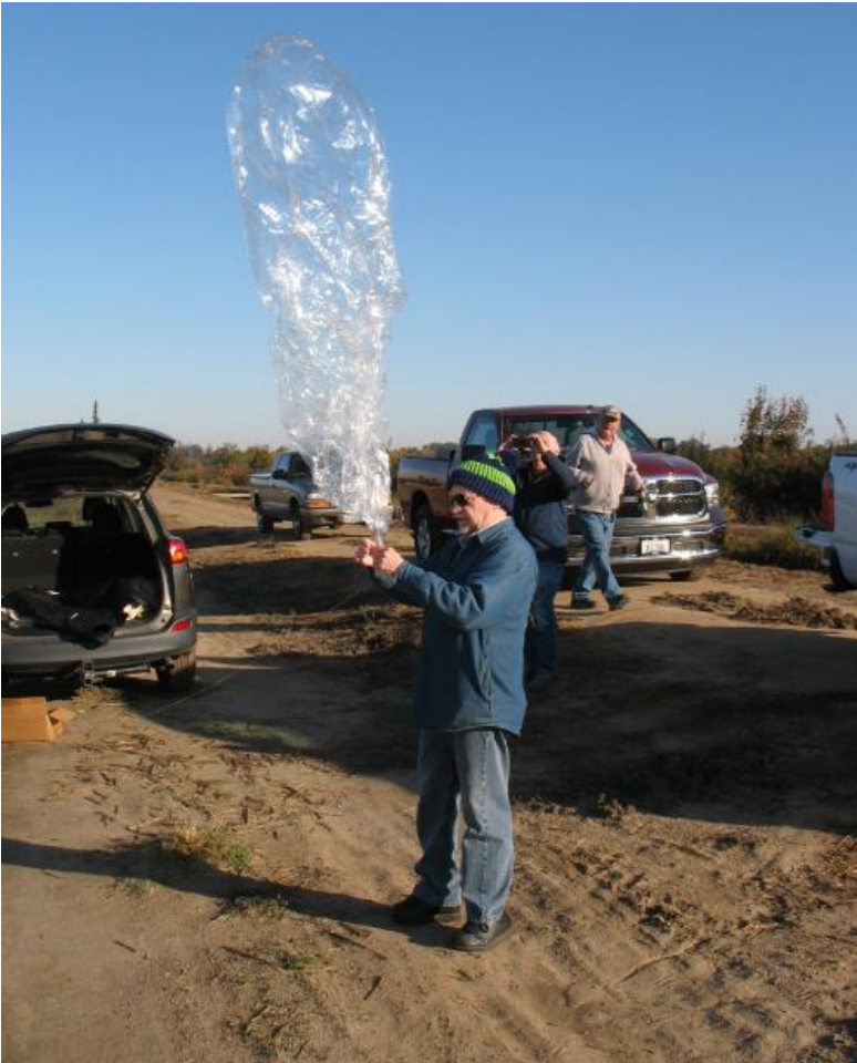
Skip prepares to release the "lifting body," the special balloon filled to a carefully calculated volume of hydrogen. WB6BET and KN6CTQ observe in the background.
