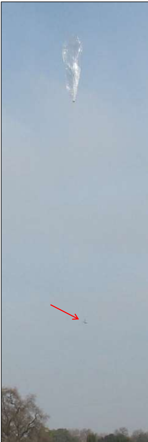
Skylarc3 rises above KM6LIA's field on January 10th. The red arrow points to the payload, trailing below at the center of the 20 meter dipole.
